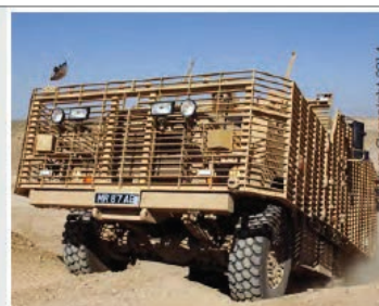
A Mastiff 3 Protected Patrol Vehicle in Helmand, Afghanistan. Mastiff is a heavily armoured, 6 x six-wheel-drive patrol vehicle which carries eight troops, plus two crew.
